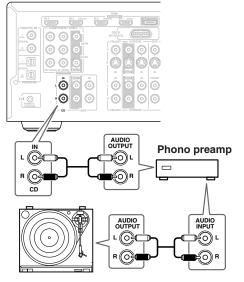
■ Turntable with an MC (Moving Coil) Cartridge
